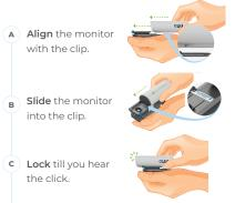
The assembled monitor should reflect the image below. The hole in the mounting clip should be aligned with the glass window on the device
